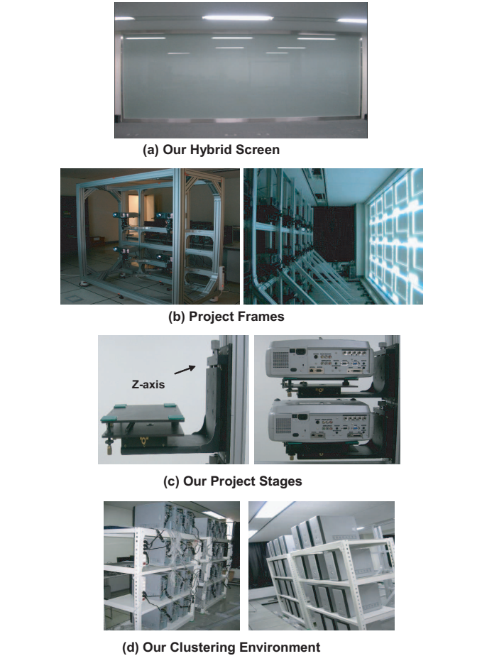
Figure 1: (a) The hybrid screen (5.6m x 2.4m size). (b) left: a typical projector frame having a box-styled design; right: our display frame - scalable, stable, easy-to-move, easy-to-use, and low-cost design. (c) Our projector stage with 6 DOF; left: a side view of our stage, right: when the stage is used for a stereo tiled display. (d) Our clustering environment for high-performance visualization using rich-featured graphics cards.
